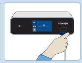
Connect the FMX Power Module to the front of the generator.
