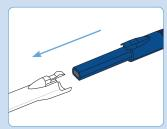
Connect the FMX Power Module to the selected FMX surgical tool. Insert the power module into the handpiece body and push until it is fully engaged.
