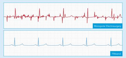
**Electromagnetic Interference:** The ECG chart to the left shows electromagnetic interference caused when using monopolar electrosurgery (top), and no interference when using the FMwand (bottom) during the same surgery.<sup>1</sup>
