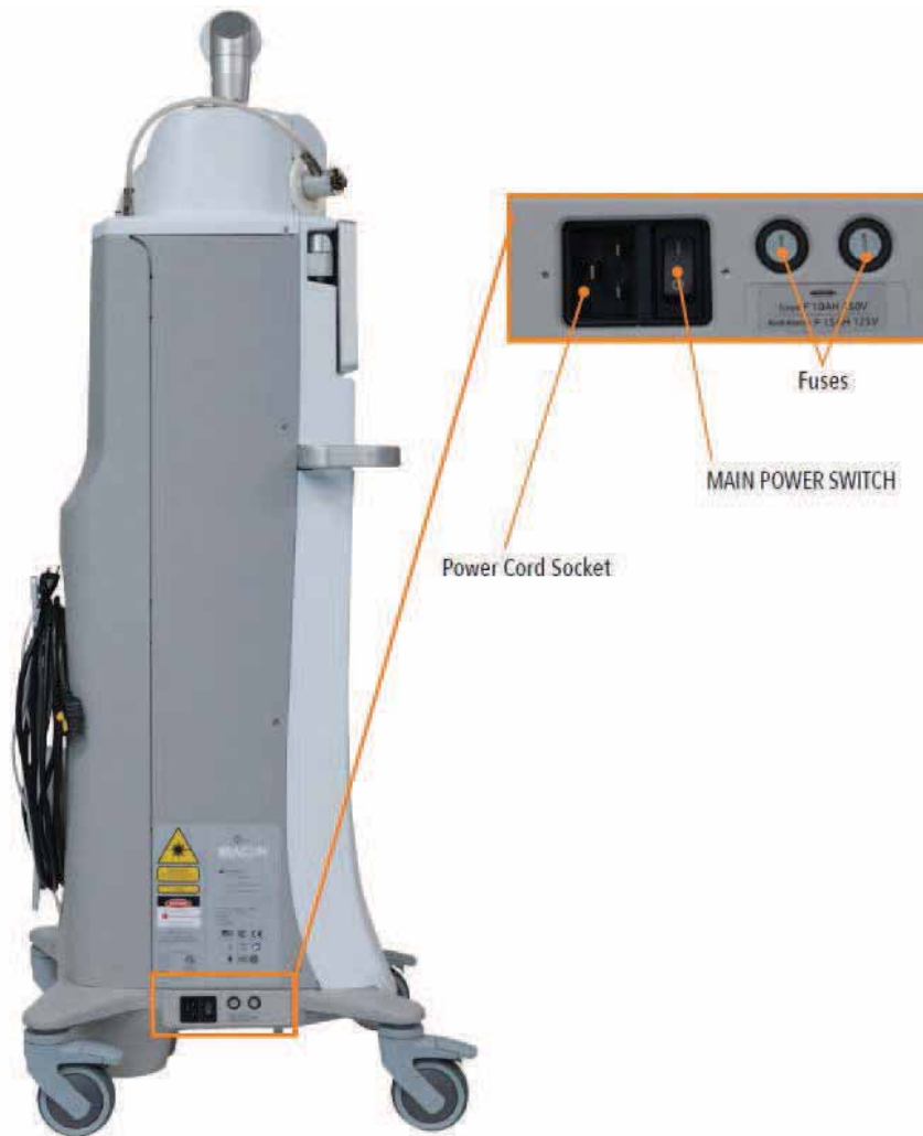
Figure 7-5. Location of the main power switch
