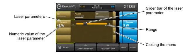
Fig. 29: Setting of the laser parameters; here in CW mode
