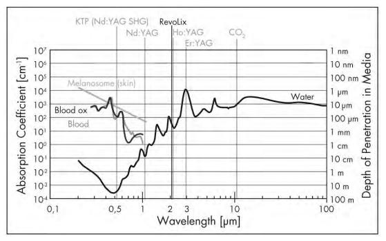
Fig. 54: Absorption spectrum of water and laser wavelengths
