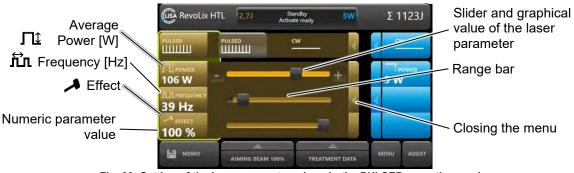
Fig. 30: Setting of the laser parameters; here in the PULSED operating mode
