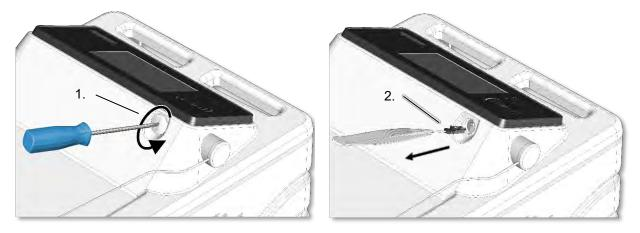
Fig. 56: Removal of the fiber coupler shield
