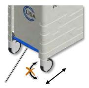
Position C Parking brake partially activated Wheels do not swivel but roll
