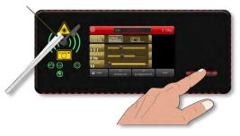
Fig. 53: Switching to the STANDBY operating state
