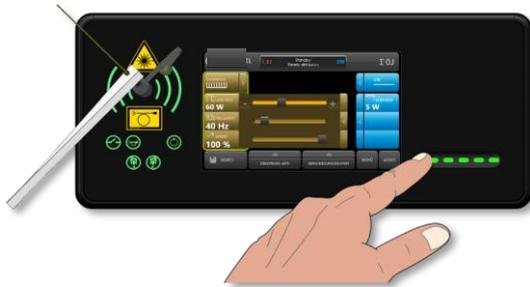
Fig. 47: Switch to LASER READY operating state
