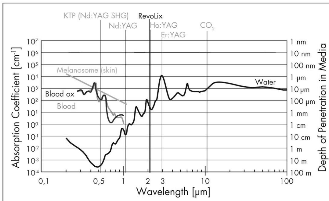
Fig. 52: Absorption spectrum of water and laser wavelengths
