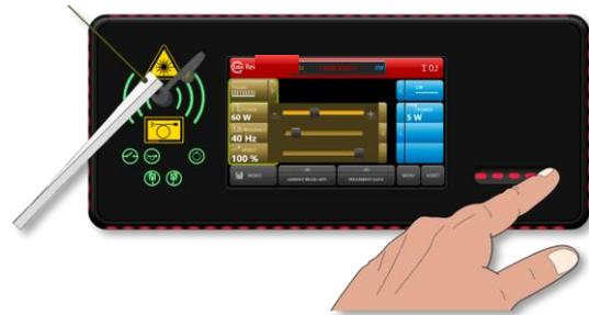
Fig. 48: Active laser warning light ribbon in LASER READY state
