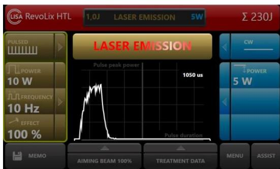
Fig. 29: Pulse shape of a short laser pulse with a high pulse peak power
