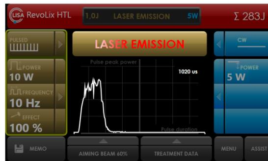
Fig. 50: Display of the laser pulse shape
