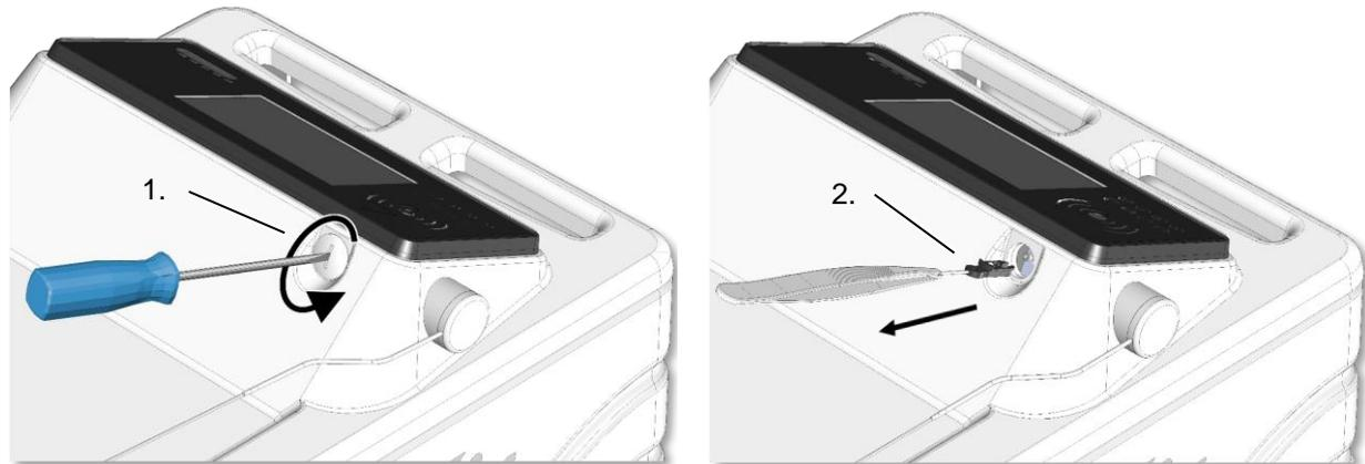
Fig. 54: Removal of the fibre coupler shield
