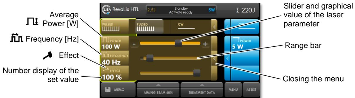
Fig. 28: Setting of the laser parameters; here in the PULSED operating mode
