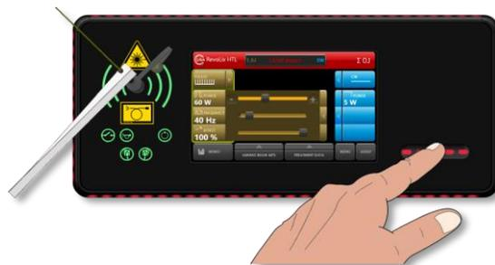
Fig. 51: Switching to the STANDBY operating state
