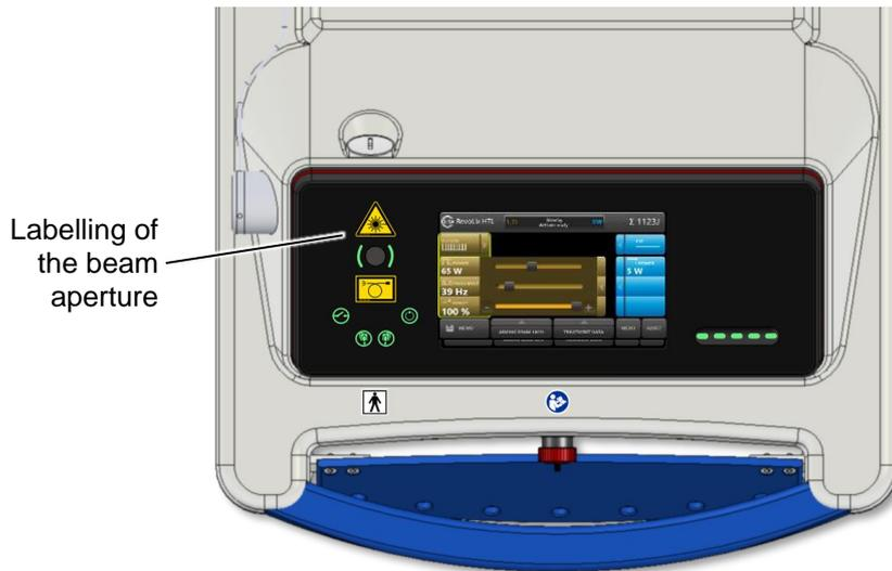
Fig. 22: Labels on the control console
