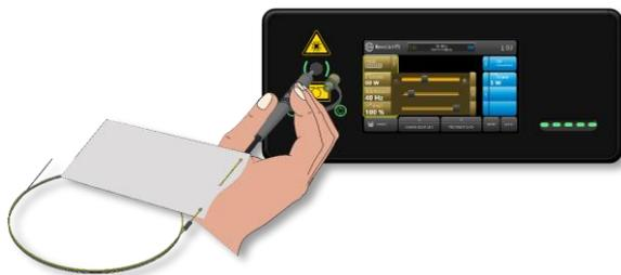
Fig. 40: Guide fibre to beam aperture
