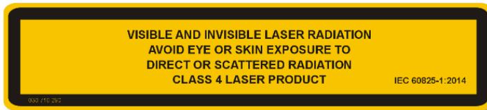
Fig. 21: Labelling of the laser class
