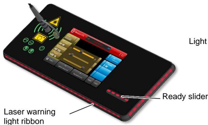
Fig. 9: Laser warning light ribbon
