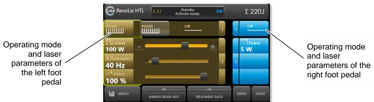
Fig. 32: Touch screen of a laser device connected to a double-pedal footswitch, left foot pedal settings are currently active
