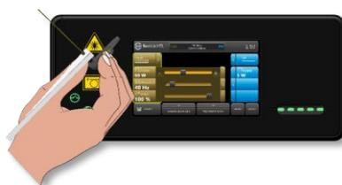
Fig. 42: Insert the fibre into the beam aperture and carefully screw it in tightly
