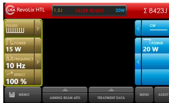
Fig. 49: The red status line indicates the LASER READY operating state
