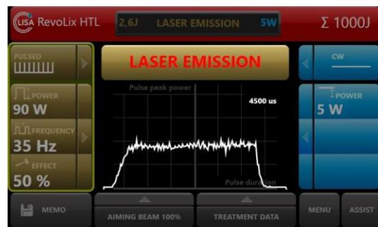
Fig. 30: Pulse shape of a long laser pulse with a low pulse peak power
