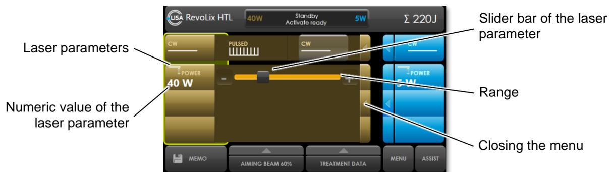
**Fig. 27: Setting of the laser parameters; here in CW mode**
