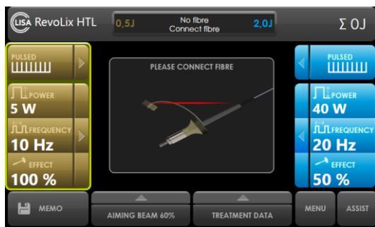
Fig. 44: Initial screen in case no RFID fibre is connected
