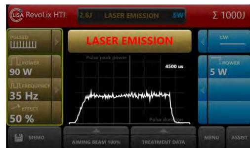
Fig. 32: Pulse shape of a long laser pulse with a low pulse peak power
