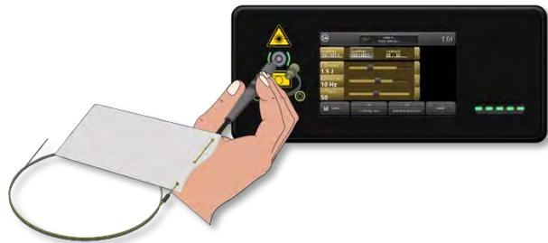
Fig. 43: Beam aperture opens automatically
