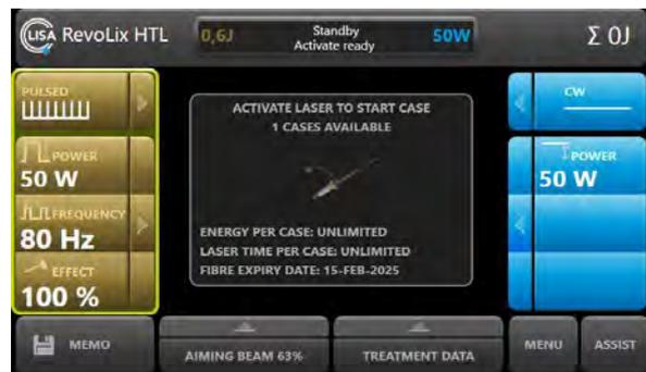
Fig. 47: Information about the connected fiber
