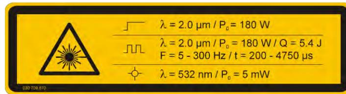
Fig. 20: Labelling of the emitted laser radiations (example – RevoLix HTL)
