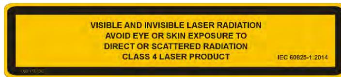
Fig. 21: Labelling of the laser class
