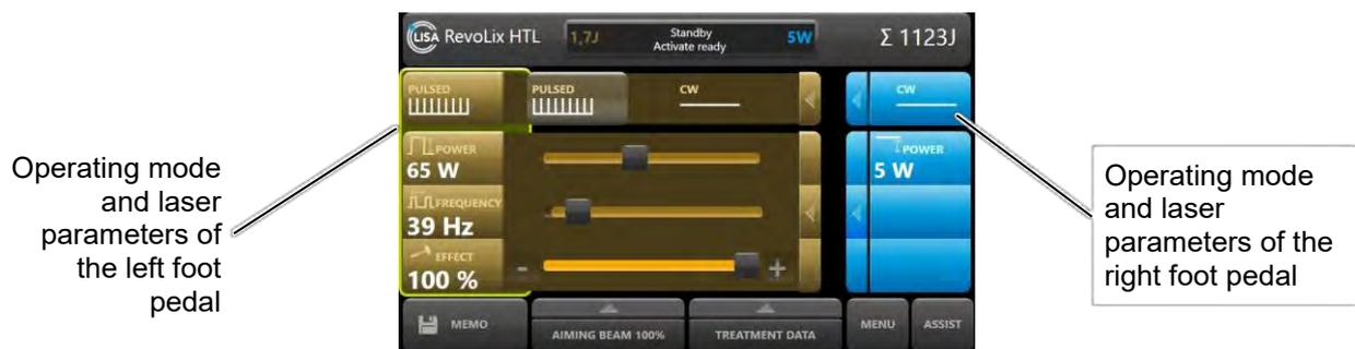
Fig. 34: Touch screen of a laser device connected to a double-pedal footswitch, left foot pedal settings are currently active
