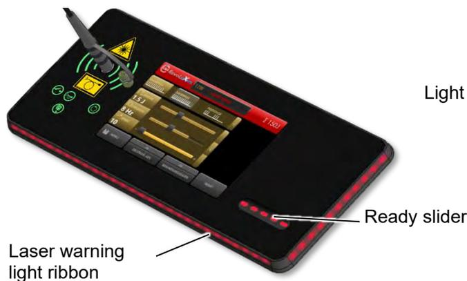
Fig. 9: Laser warning light ribbon
