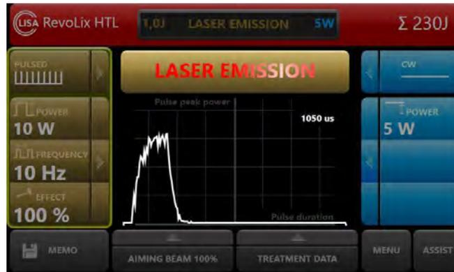
Fig. 52: Display of the laser pulse shape
