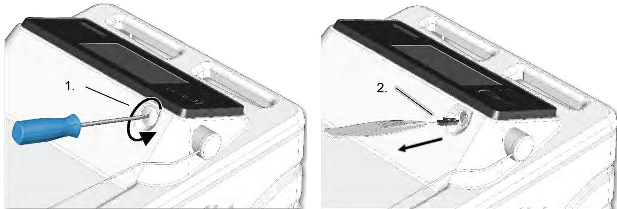
Fig. 56: Removal of the fiber coupler shield
