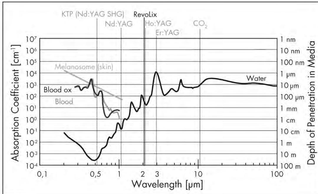
Fig. 54: Absorption spectrum of water and laser wavelengths
