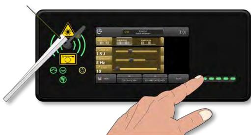
Fig. 49: Switch to LASER READY operating state
